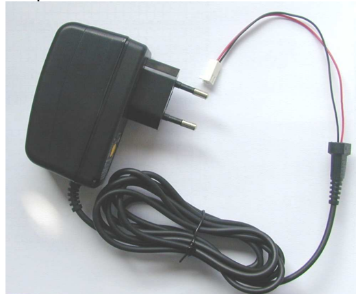
Figure 4: Power supply block
